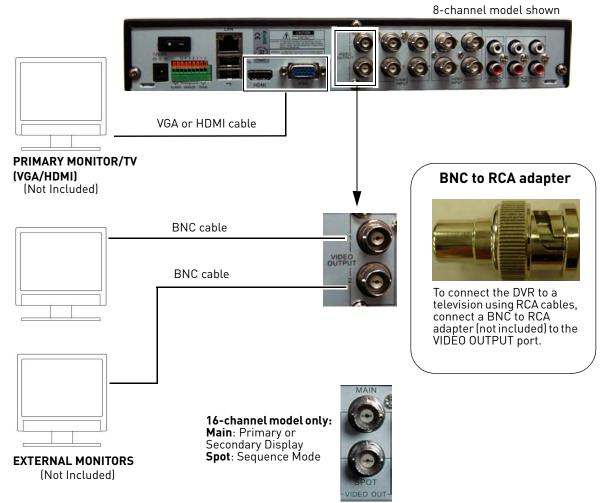
On the 16-channel model, connect external monitors to either the Main or Spot port.
